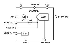
Customers desiring multichannel digitization may consider the AD9059, a dual 8-bit, 60 MSPS monolithic based on the AD9057 ADC core. The AD9059 is available in a 28-lead surface mount plastic package (28 SSOP) and is specified over the industrial temperature range.
