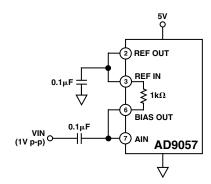
Figure 2. Capacitively Coupled AD9057
