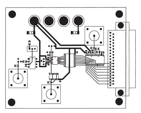
Figure 8. Evaluation Board Layout
