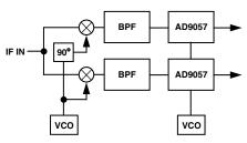
Figure 4. I and Q Digital Receiver
