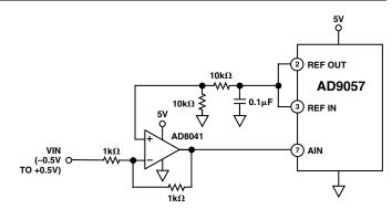
Figure 3. DC-Coupled AD9057 (Inverted VIN)
