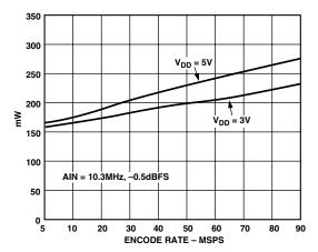
TPC 7. Power Dissipation vs. Encode Rate
