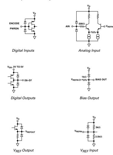
Figure 6. Equivalent Circuits
