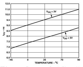
TPC 10.  $t_{PD}$  vs. Temperature/Supply ( $V_{DD} = 3 \text{ V/5 V}$ )
